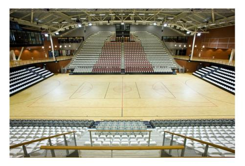
The floor is a floating wooden floor, type multilastic triathlon KH. The surface area is at least 45 x 25 meters.
